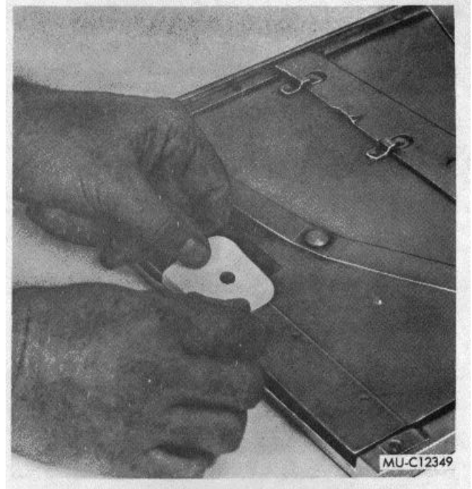
Figure 2-11. Fastening table to button.
